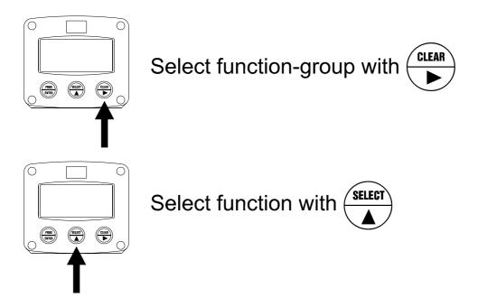
Each function has a unique number, which is displayed below the word "SETUP" at the bottom of the display. The number is a combination of two figures. The first figure indicates the function-group and the second figure the sub-function. Additionally, each function is expressed with a keyword.
