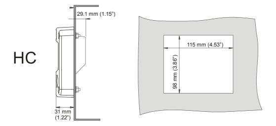
Fig. 5: Dimensions GRP enclosures.
