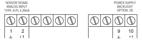
Fig. 6: Overview of terminal connectors standard configuration F090-A-PL and options.
