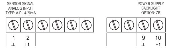
Fig. 9: Overview terminal connectors XI - Intrinsically Safe applications.
