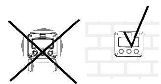
Mount the F090-A-PL on a solid structure to avoid vibrations.
