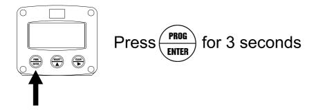
In order to return to the operator level, PROG will have to be pressed for three seconds. Also, when no keys are pressed for 2 minutes, SETUP will be left automatically.
