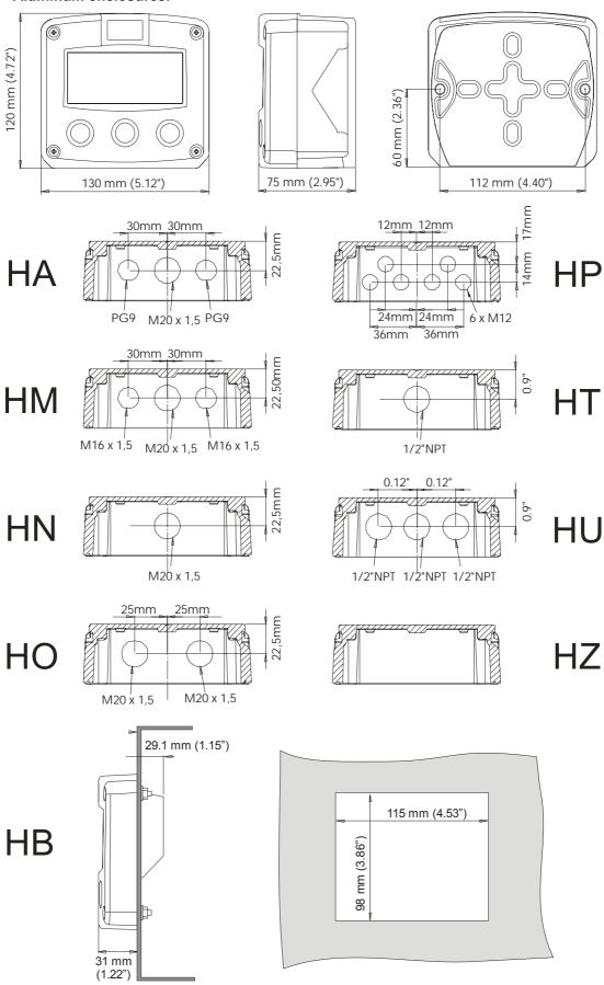
Fig. 4: Dimensions Aluminum enclosures.
